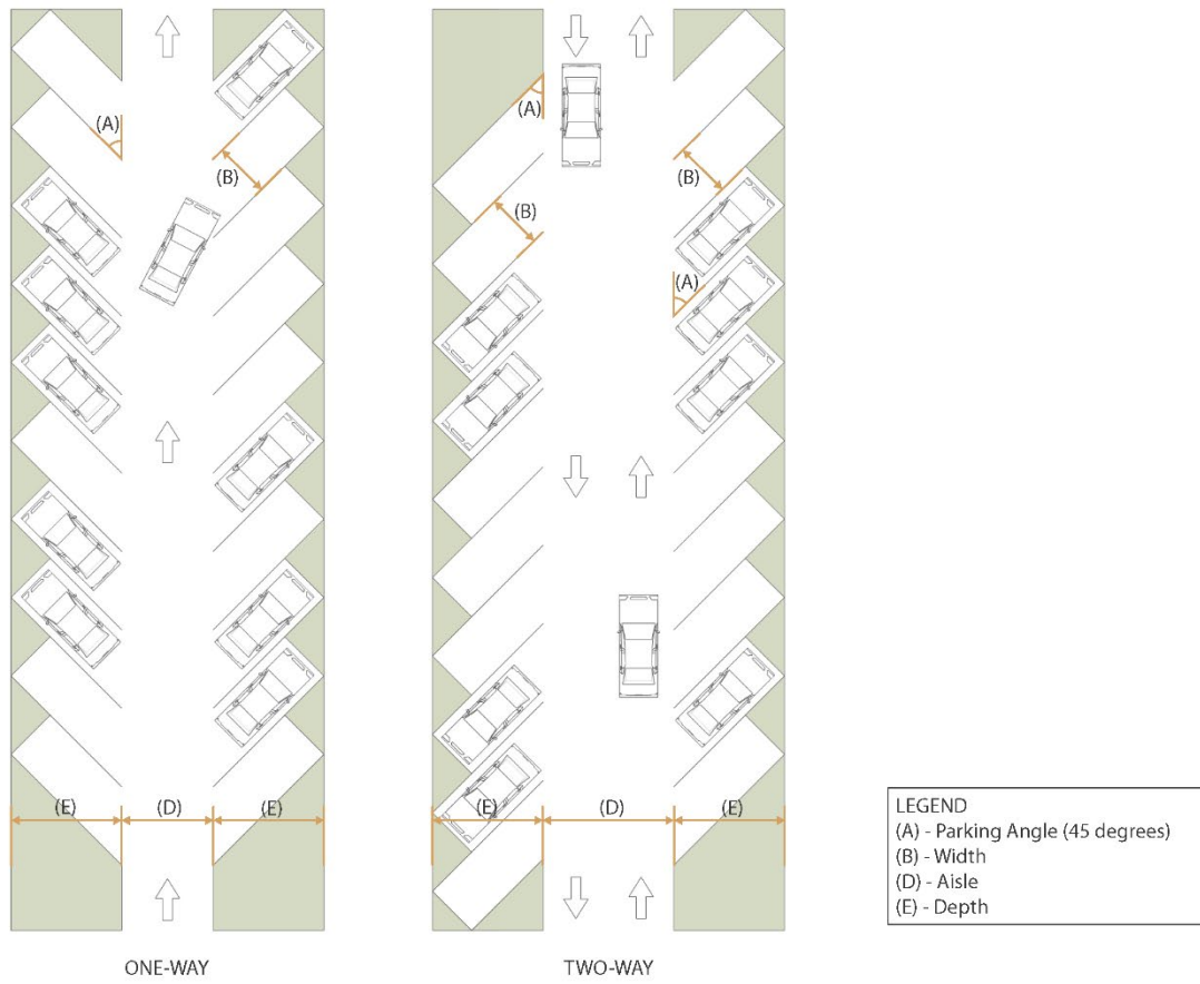
Figure 15.6.1 – Parking Angle: 45 Degrees.
