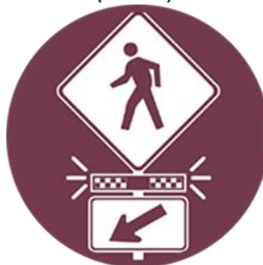
Rectangular Rapid Flashing Beacons (RRFB)
