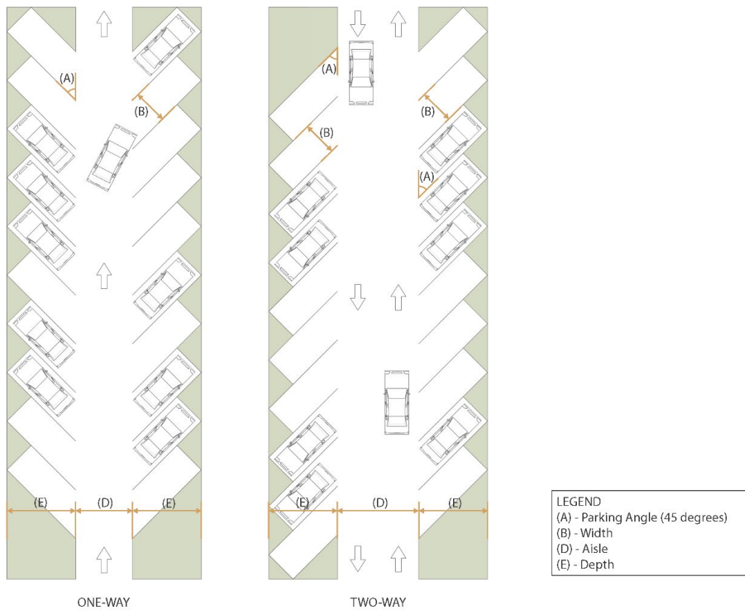
Figure 15.6.1 – Parking Angle: 45 Degrees.
