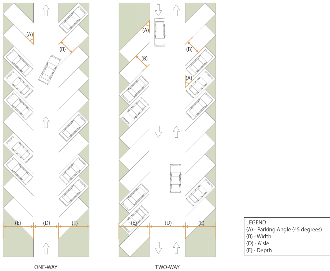
Figure 15.6.1 – Parking Angle: 45 Degrees.
