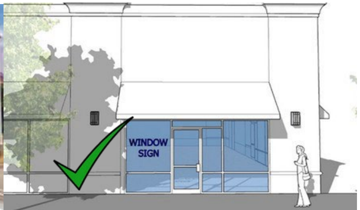
Signage is within 30% window coverage
